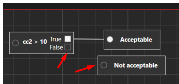
Figure 7.163 Conditional node with connected “Acceptable” result node
